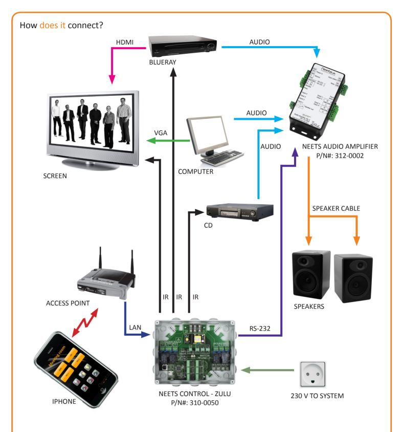
The Neets Control - ZULU is controlling the screen, blueray and CD player via IR. The Neets Audio Amplifier is controlled from the RS-232 port on the control system. Through the access point which is connected to the control system via LAN, the IPhone, IPad or other touch panel with web browser, is controlling the system. Audio signals from the blueray, computer and the CD player is is connected to the Neets Audio Amplifier.
